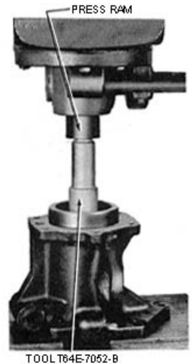
Figure 11 – Installing Adapter Housing Seal
